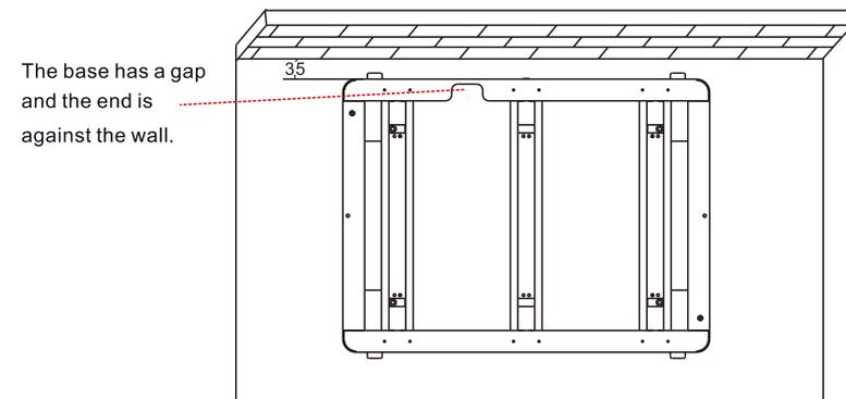
**Step 5:** Use wall mounted positioning cardboard, and mark the holes layer by layer.
