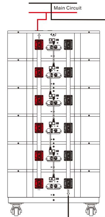
The diagram of six battery strings in parallel is shown in the figure above. In order to maintain the current balance of the battery pack, please ensure that the negative electrode of the battery comes out from the bottom.
