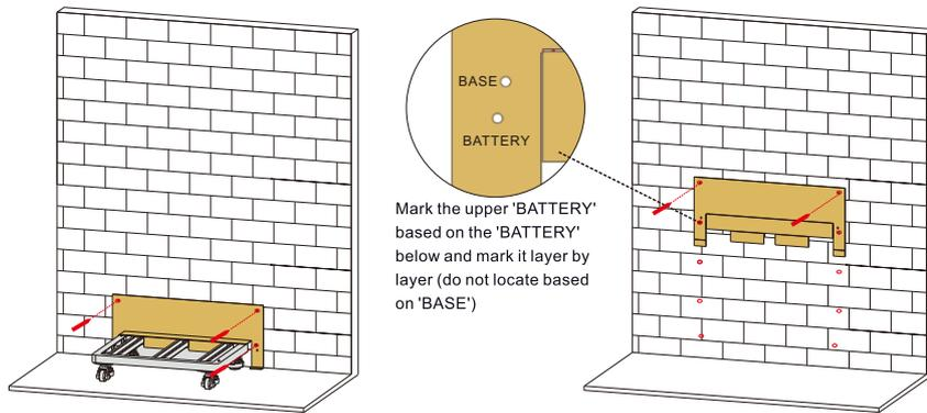
Mark the upper 'BATTERY' based on the 'BATTERY' below and mark it layer by layer (do not locate based on 'BASE')
