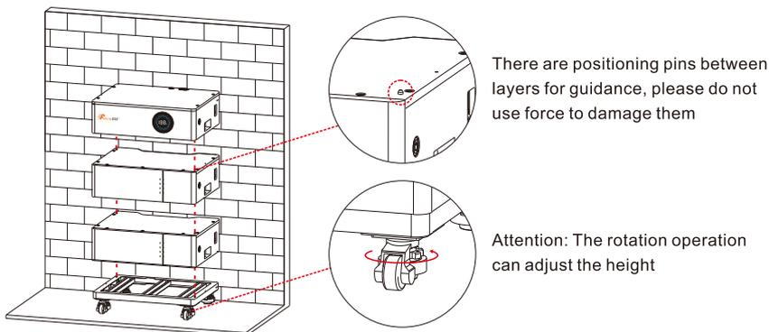
There are positioning pins between layers for guidance, please do not use force to damage them
