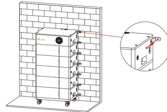
The battery packaging layer is fixed between the layers using hexagonal screws (at the handle)
